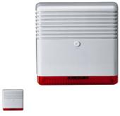
Outdoor, Tampering Protected Siren SIR/PL Outdoor siren with flasher ; Acoustic pressure: 120 dB @1 m; Tamper switch contact: 1A/ 12V ; Flash lamp: High Bright LED ; Operating voltage: 11 – 14 V DC ; Stand by current drain: 10 mA ; UV protected, polycarbonate plastic box
